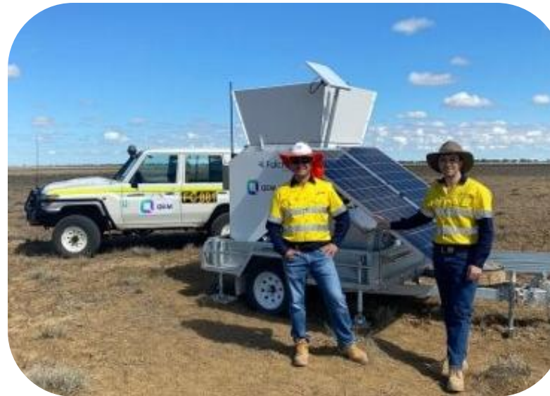
SODAR & LiDAR equipment installed on site at Julia Creek
